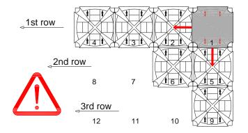
Before starting to install the elements, we recommend that you consult Geoplast® project tables to position the elements appropriately. For a correct installation, in compliance with safety regulations, please refer to the installation manual.
