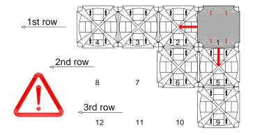
Before starting to install the elements, we recommend that you consult Geoplast® project tables to position the elements appropriately. For a correct installation, in compliance with safety regulations, please refer to the installation manual.
