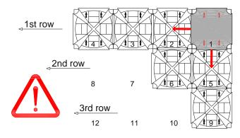
Before starting to install the elements, we recommend that you consult Geoplast® project tables to position the elements appropriately. For a correct installation, in compliance with safety regulations, please refer to the installation manual.
