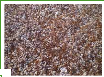
PERMEABLE SUB-BASE 10 - 15 cm
