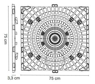
$^{\ast}$  in consideration of the recycled material the measurements must be considered with a tolerance of  $\pm$  1.5%.
