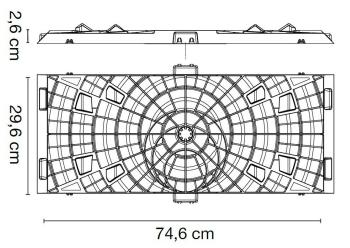
\* in consideration of the recycled material the measurements must be considered with a tolerance of ± 1.5%.
