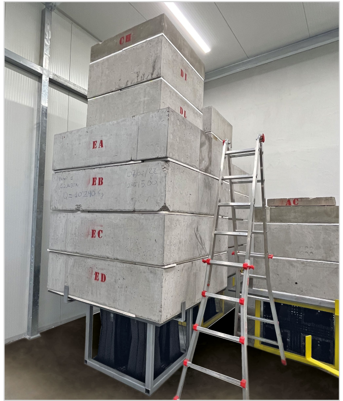
Aquabox load test concrete specimens
