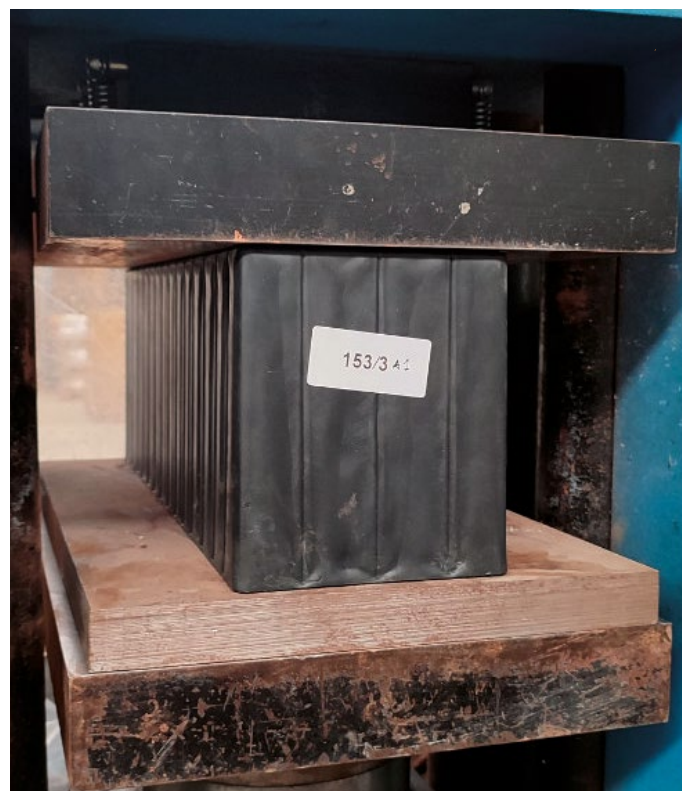
Strength test of the new polypropylene element
